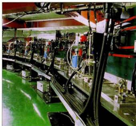
The damping ring at the Accelerator Test Facility (ATF) at the Japanese KEK laboratory has attained promising beam emittances (size \times divergence) for new electron-positron linear colliders.
