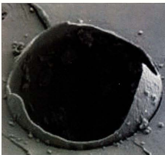
Above left, top right: scanning electron micrographs of a ruptured capsule on its way to mending the surrounding polymer. Bottom right: self-healing polymers in action, as seen by a scanning electron microscope. The ruptured capsule is red; the fracture plane is light blue. The chemical structure appearing to emerge from the capsule is the polymerized healing agent. The other chemical structure in several colours is that of the catalyst.
