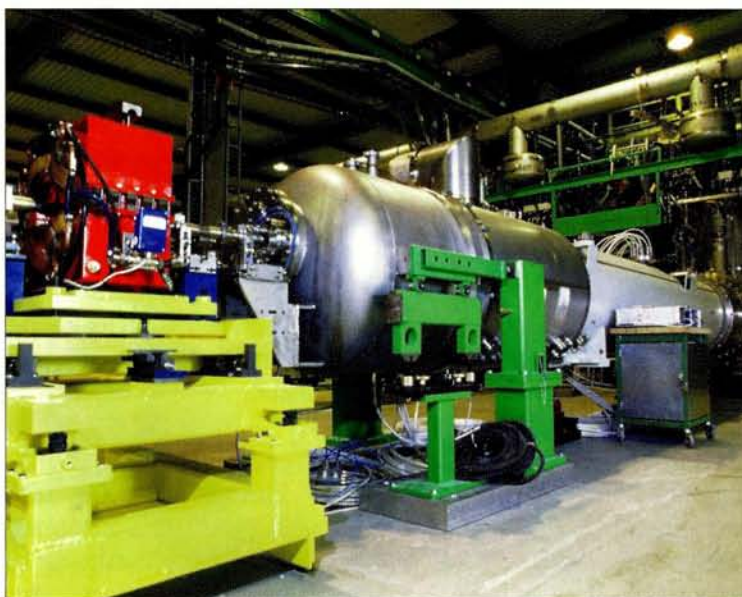
A short straight section, containing a prototype LHC main quadrupole, on its testbench at CERN.
