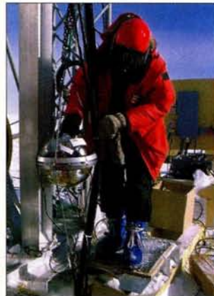
Left: an optical module of the AMANDA neutrino detector being lowering into the Antarctic ice. Right: physics under Antarctic conditions – deploying a photomultiplier at AMANDA.
