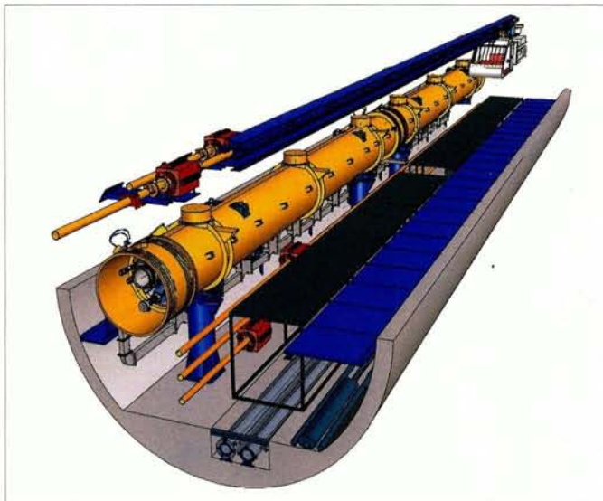
How TESLA will look – the yellow cryostats conceal the superconducting niobium cavities for particle acceleration, which operate at -271^{\circ}\text{C} .
