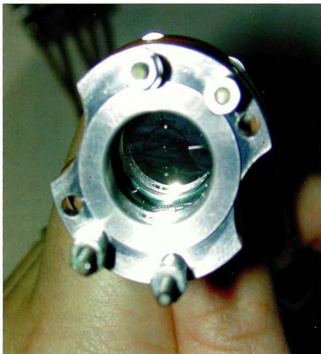
A thin silicon sensor (67 \mu\text{m} thick) used as a beam counter for antiprotons at the ATHENA experiment at CERN (P Riedler, Zürich). The counter is installed in vacuum at 10 K and a magnetic field of 3 T.
