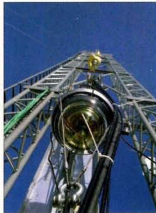
Left: an optical module of the AMANDA neutrino detector being lowering into the Antarctic ice. Right: physics under Antarctic conditions – deploying a photomultiplier at AMANDA.
